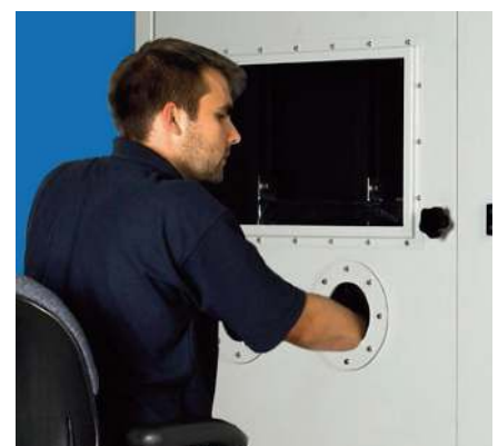
Instrument access via airtight gauntlets and viewing panel
