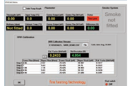
The software interfaces with the OSU apparatus via a data logger system, into which all the required signals are connected
