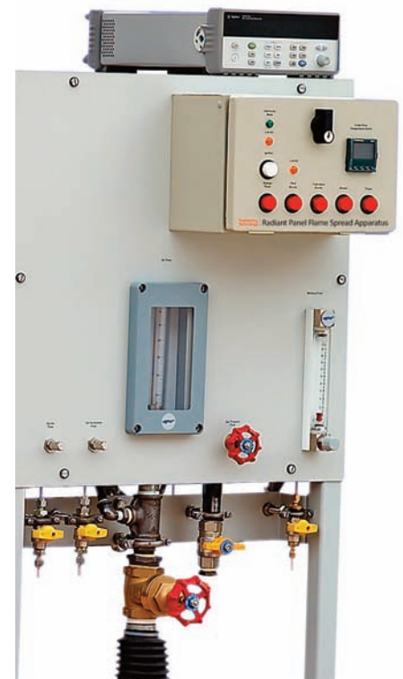
Gas Panel, Control Box and Data Logger
