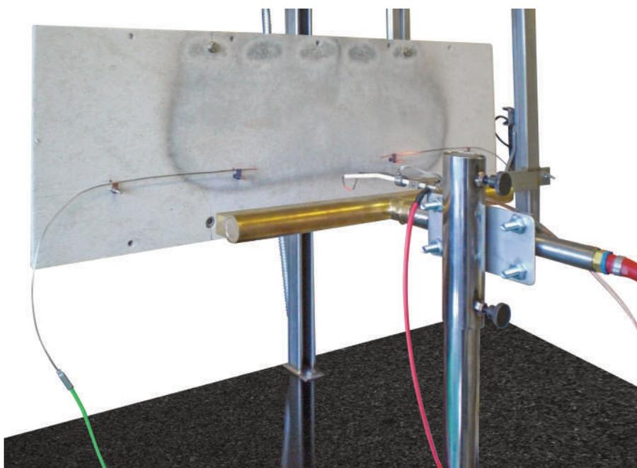
Resistance to Fire with Mechanical Shock
