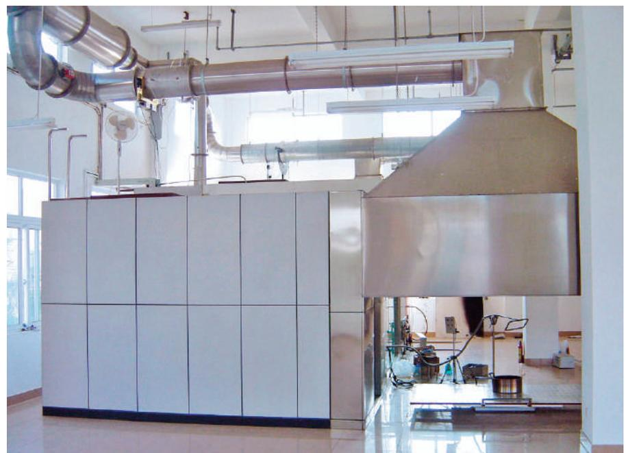
Figure 2: **FTT** ISO 9705-2 Large Scale Calorimeter with Weight Measurement (Room chamber on left not included in standard configuration)
