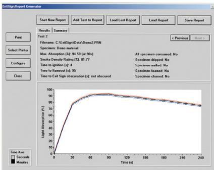
horizontally across the 300mm (12") light beam path. The chamber is closed during the 4 minute test period except for the 25mm (1") high ventilation openings around the bottom of the chamber.
