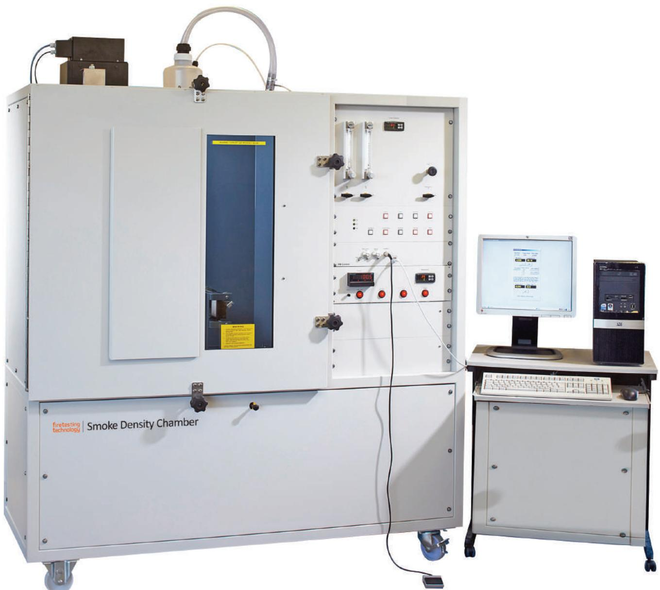
Figure 11: FTT Smoke Density Chamber
