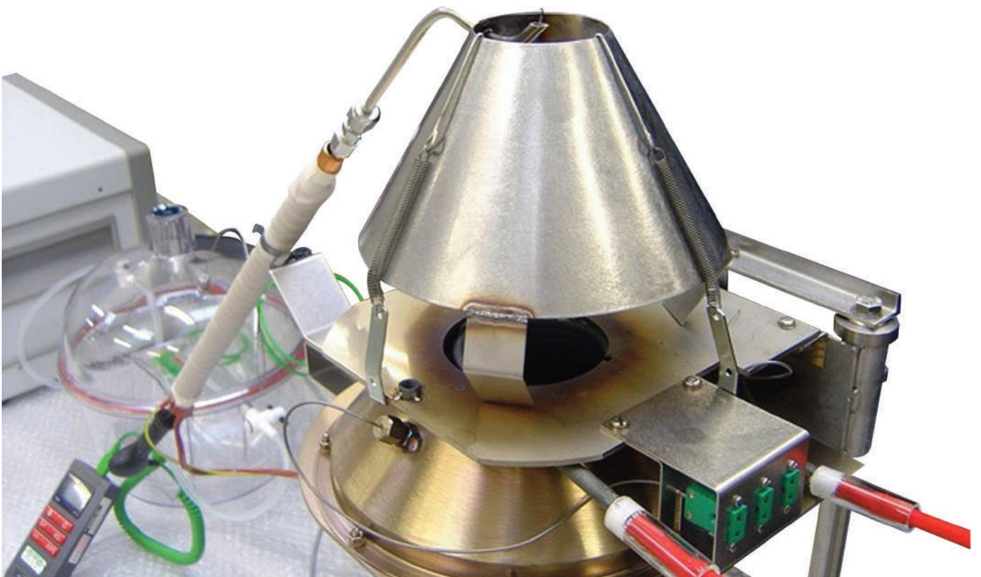
The Cone Calorimeter and Mass Loss Calorimeter can be used to determine the corrosive effect of combustion products when used with a cone corrosimeter.
