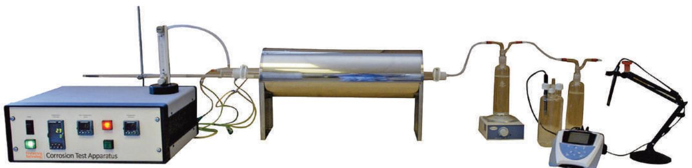
The International Electrotechnical Commission IEC 60754 Part 1 and Part 2 test is performed to determine the degree of acidity of gases evolved during the combustion of materials taken from electric cables by measuring the pH and conductivity.
