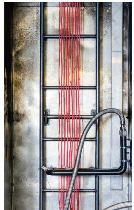
EN 50399 Cable Test Interior detail
