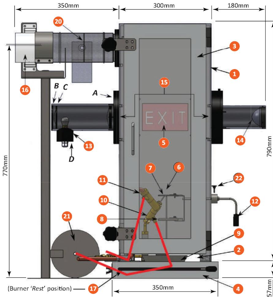
1. Combustion Chamber: 300mm × 300mm × 790mm
