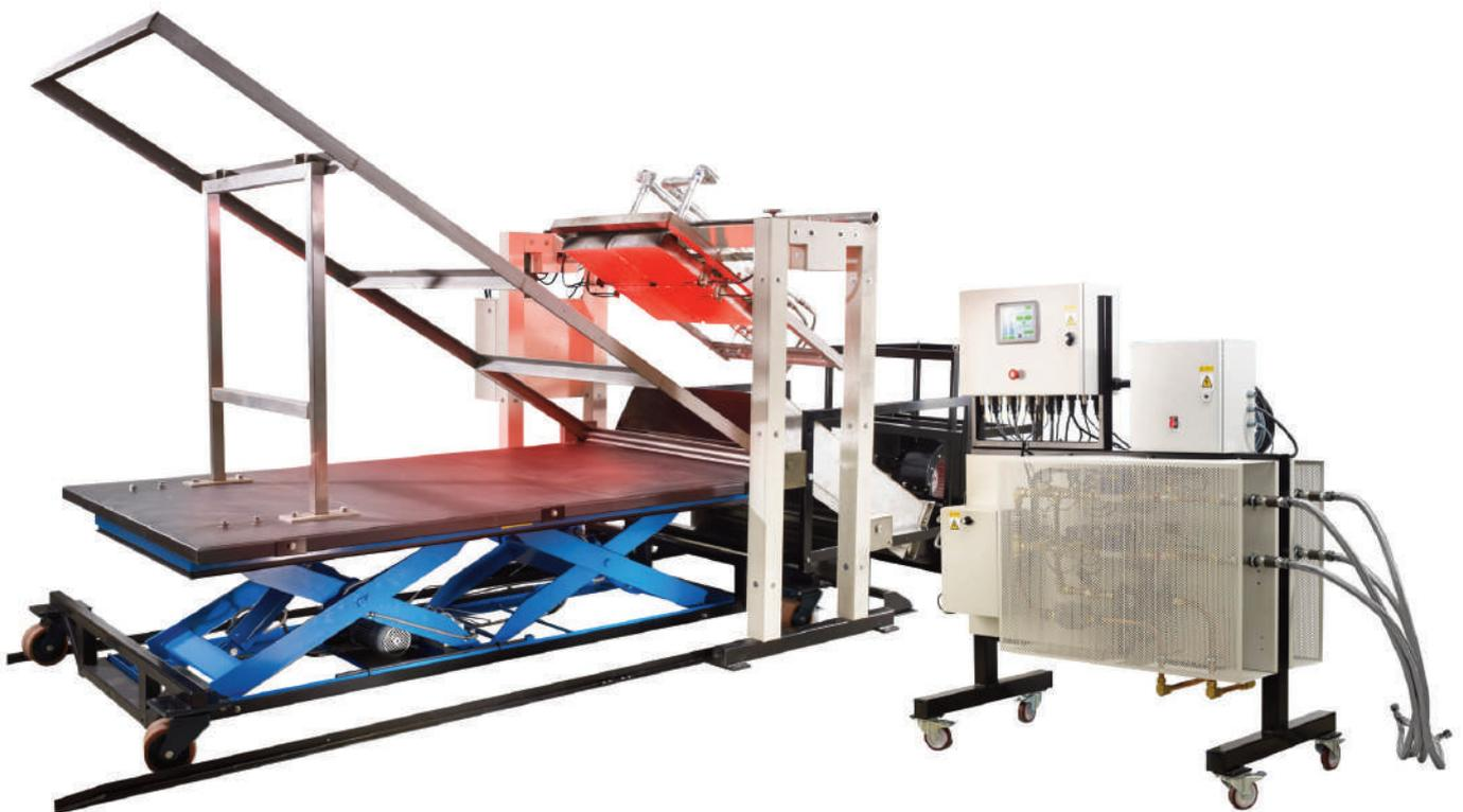
This **ENV 1187** describes four methods for determining the performance of roofs to external fire exposure. The four methods assess the performance of roofs under the following condition
