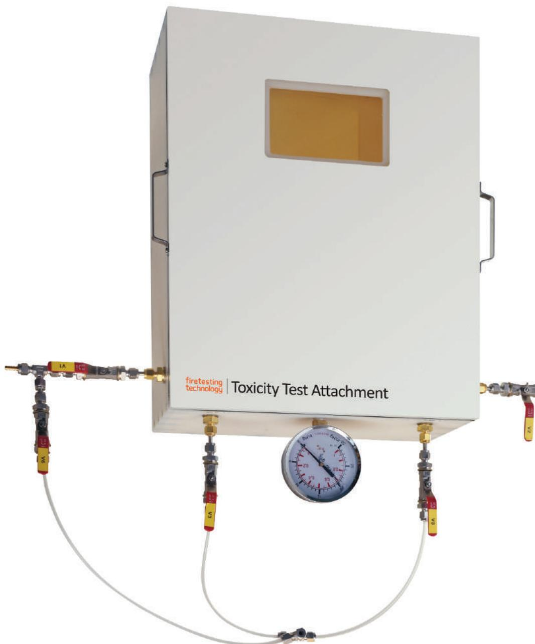
Using in conjunction with the NBS Smoke Density Chamber, gaseous/volatile test products are drawn from the chamber at any time for analysis through three ports on the top of the chamber. One of these ports is used to connect to the ABD0031 vacuum box.
