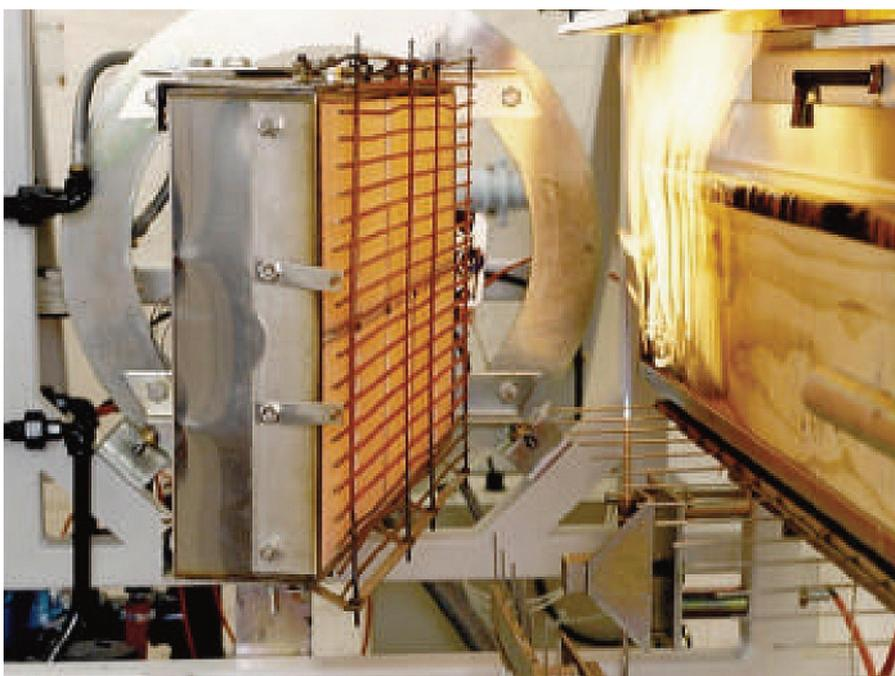
Panel box assembly with reverberatory screen as mounted in equipment test frame.
