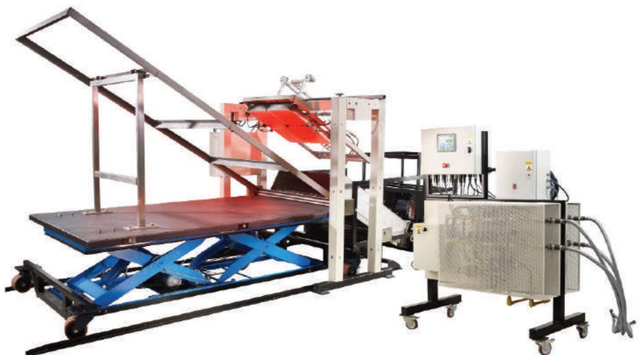
detailed in the standard. The volume flow rate of the blower is controlled via the Touch Screen interface on the Diverter Stand.
