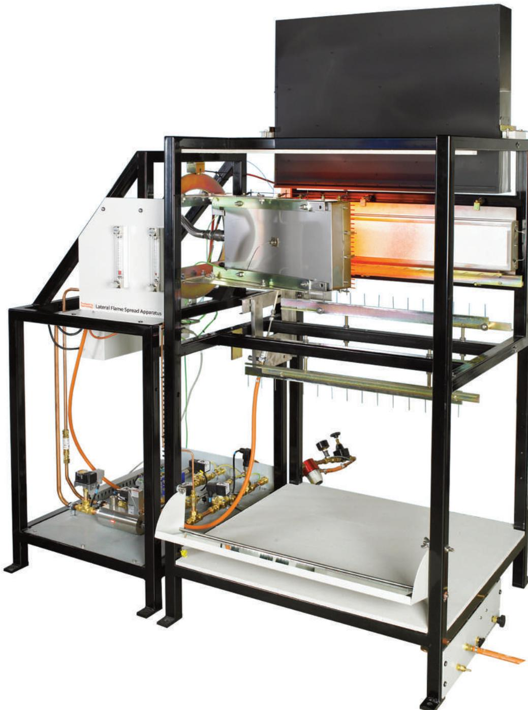
The Spread of Flame Apparatus is an important test for comparing the performance of essentially flat materials, composites or assemblies, which are used primarily as the exposed surfaces of walls. Comparative test data is generated from measurement of the lateral spread of flame along the surface of a specimen of a product vertically orientated. The specimen is subject to radiated heat in the presence of a pilot flame.
