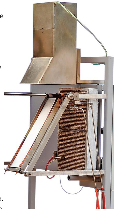
Radiant Panel, Specimen Holder and Exhaust Stack
