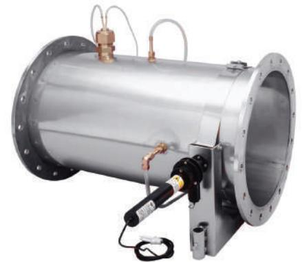
Duct section placed in EN 50399 exhaust
