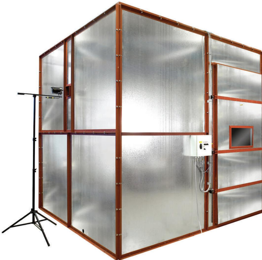
Figure 13: **FTT** EN 61034 3M Cube Smoke Test Apparatus
