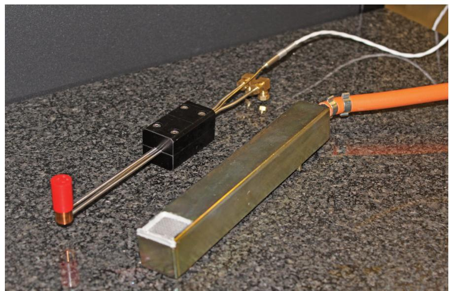
Heat flux meter and calibration burner
