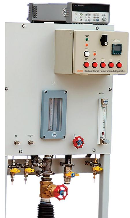
Gas Panel, Control Box and Data Logger
