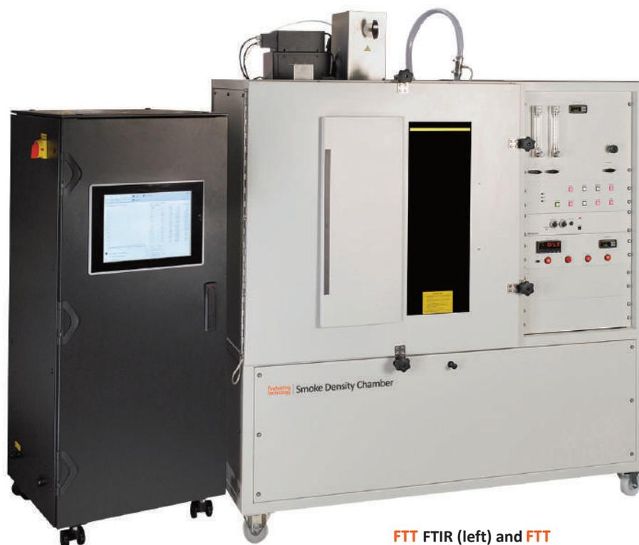
**FTT FTIR (left) and FTT Smoke Density Chamber (right)**
