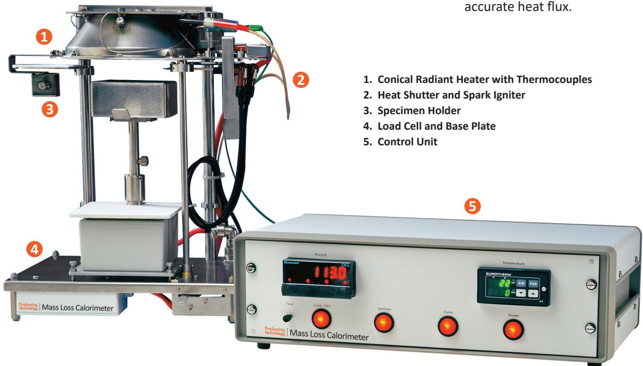
1. Conical Radiant Heater with Thermocouples
