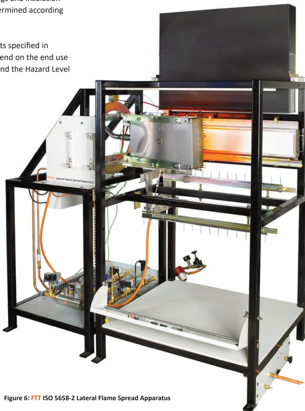
Figure 6: FTI ISO 5658-2 Lateral Flame Spread Apparatus
