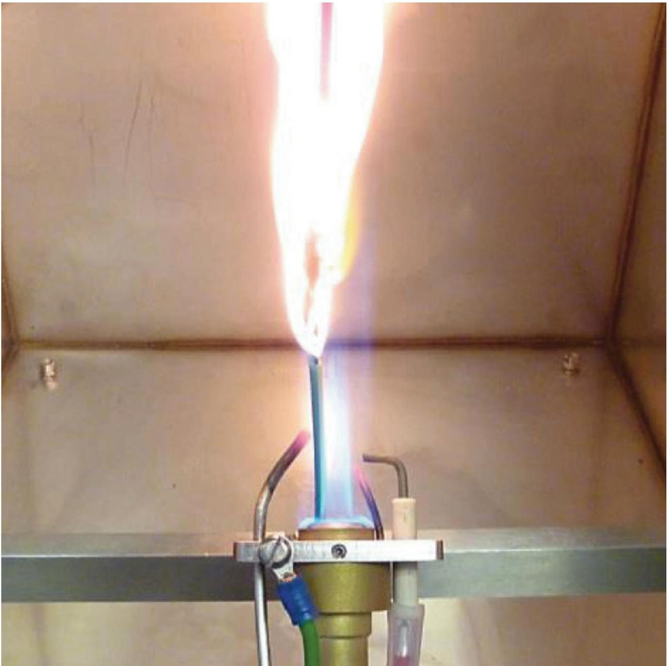
**IEC 60332-1:****Tests on electric and optical fibre cables under fire conditions**
