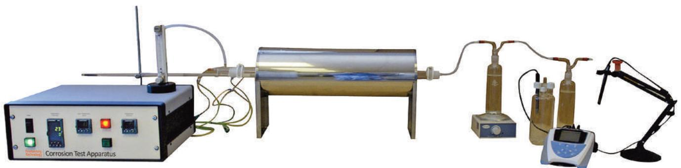
Figure 12: FTT NF X 70-100-2 / EN 50267-2-3 Toxicity Test
