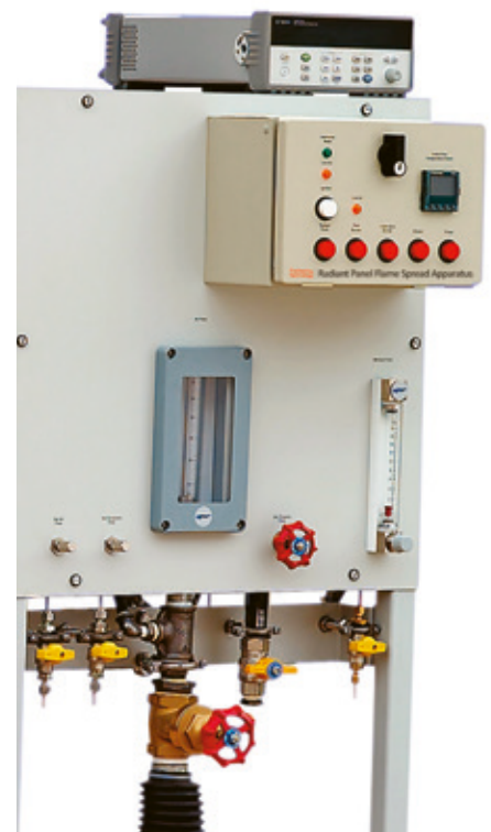
Gas Panel, Control Box and Data Logger
