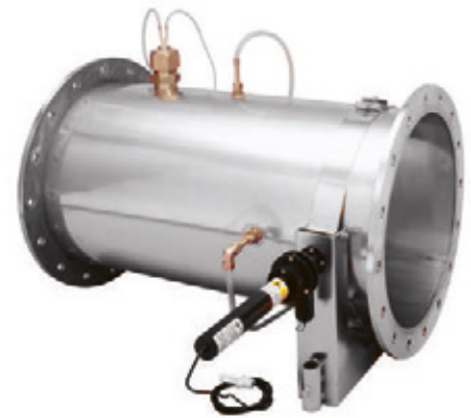
Duct section placed in EN 50399 exhaust
