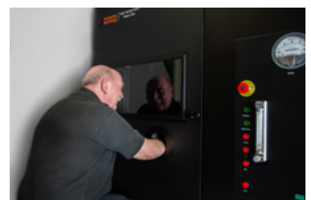
Instrument access via airtight gauntlets and viewing panel
