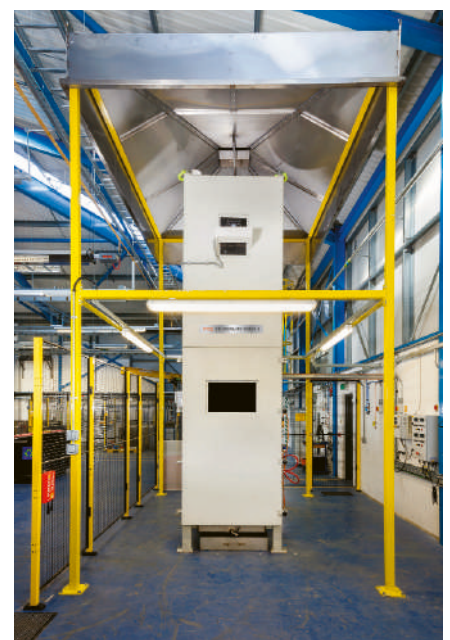
Front view of cable test chamber and hood
