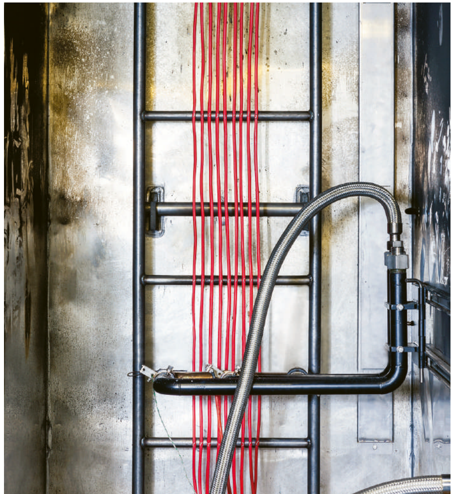
Test chamber interior detail with propane burner
