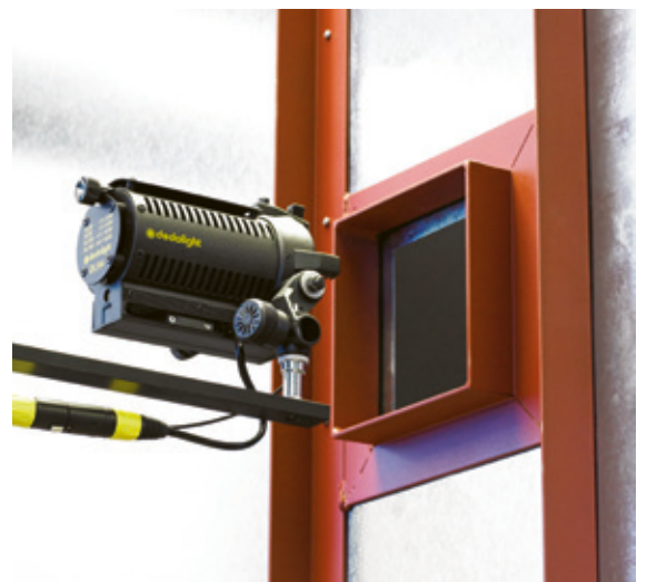
Detail of light source and detector at opposing apertures
