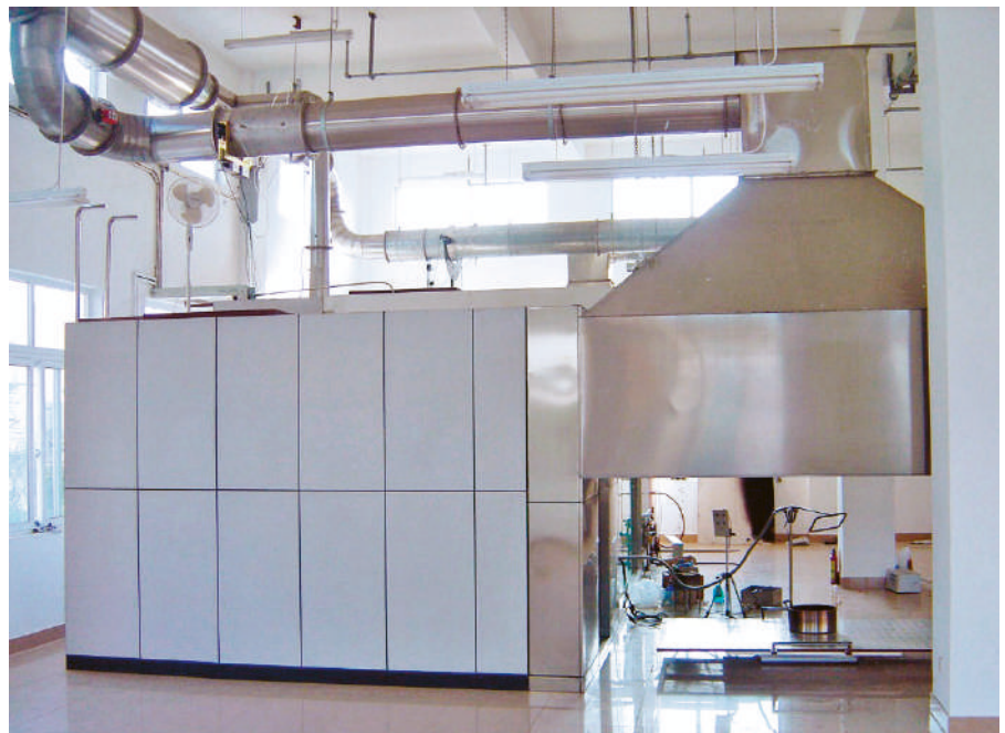
Figure 2: FTT ISO 9705-2 Large Scale Calorimeter with Weight Measurement (Room chamber on left not included in standard configuration)
