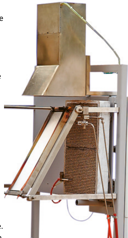
Radiant Panel, Specimen Holder and Exhaust Stack
